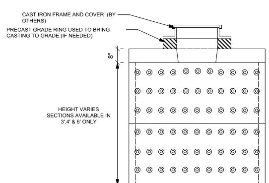
5000 PSI CONCRETE @ 28 DAYS REINFORCING GRADE 60 H-20 LOADING
