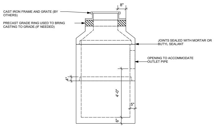
5000 PSI CONCRETE @ 28 DAYS MANUFACTURED TO MEET OR EXCEED ASTM SPEC C-478. HS-20 LOADING OPENINGS CAST AT REQUIRED LOCATIONS
